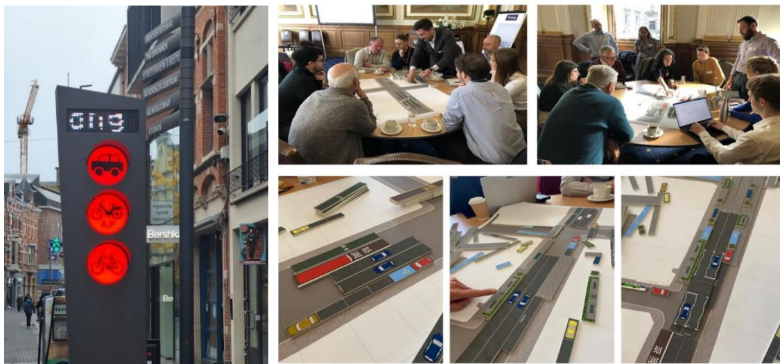
Figure 12. 'Traffic lights' in Leuven communicate which modes are not permitted at that time and is updated during the day automatically (left, source: author). An interactive tool for engaging stakeholders with street-space allocation (right, source: Edinburgh)
