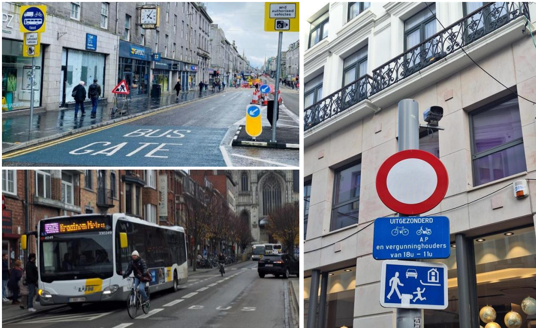
Figure 9. Aberdeen's bus gates use ANPR, signage and road markings (top left source: BBC). In Leuven, ANPR is used with signage to open up space on pedestrian streets (right) and those with buses (bottom, left). ANPR can be applied very flexibly to streets (source: author)
