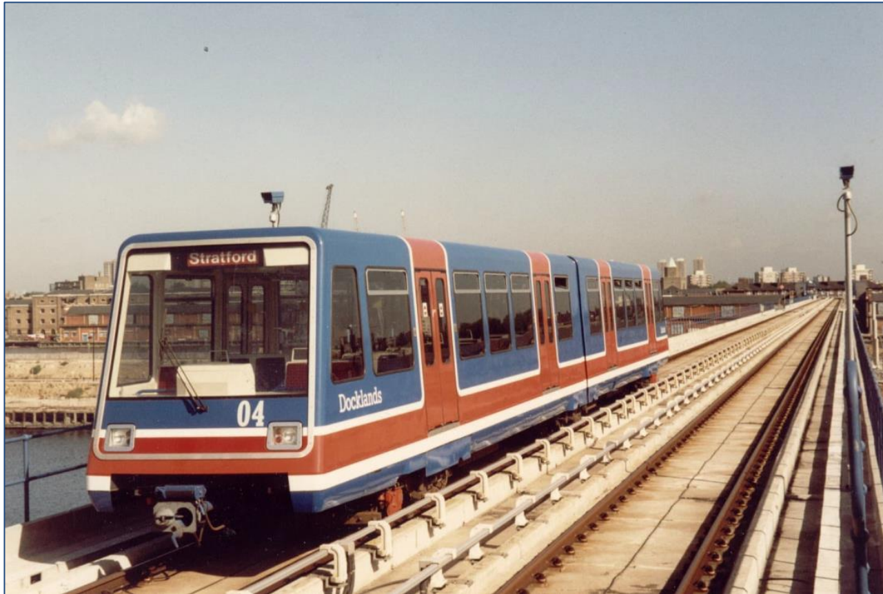
Docklands Light Rail (DLR) has been operating with fully driverless technology since 1987
